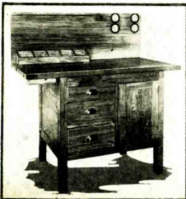
The work bench rearranged for the use of the Service Man; the radiotician's tools replace the carpenter's. The Jewell meters shown are: one A.C. "Model 78," 0-3-15-150-volt reading; and three D.C. "Model 88" with these scales—0-15-150 ma. and 0-75-volt; 0-1-10-amp.; and 0-150-300-750-volt.
